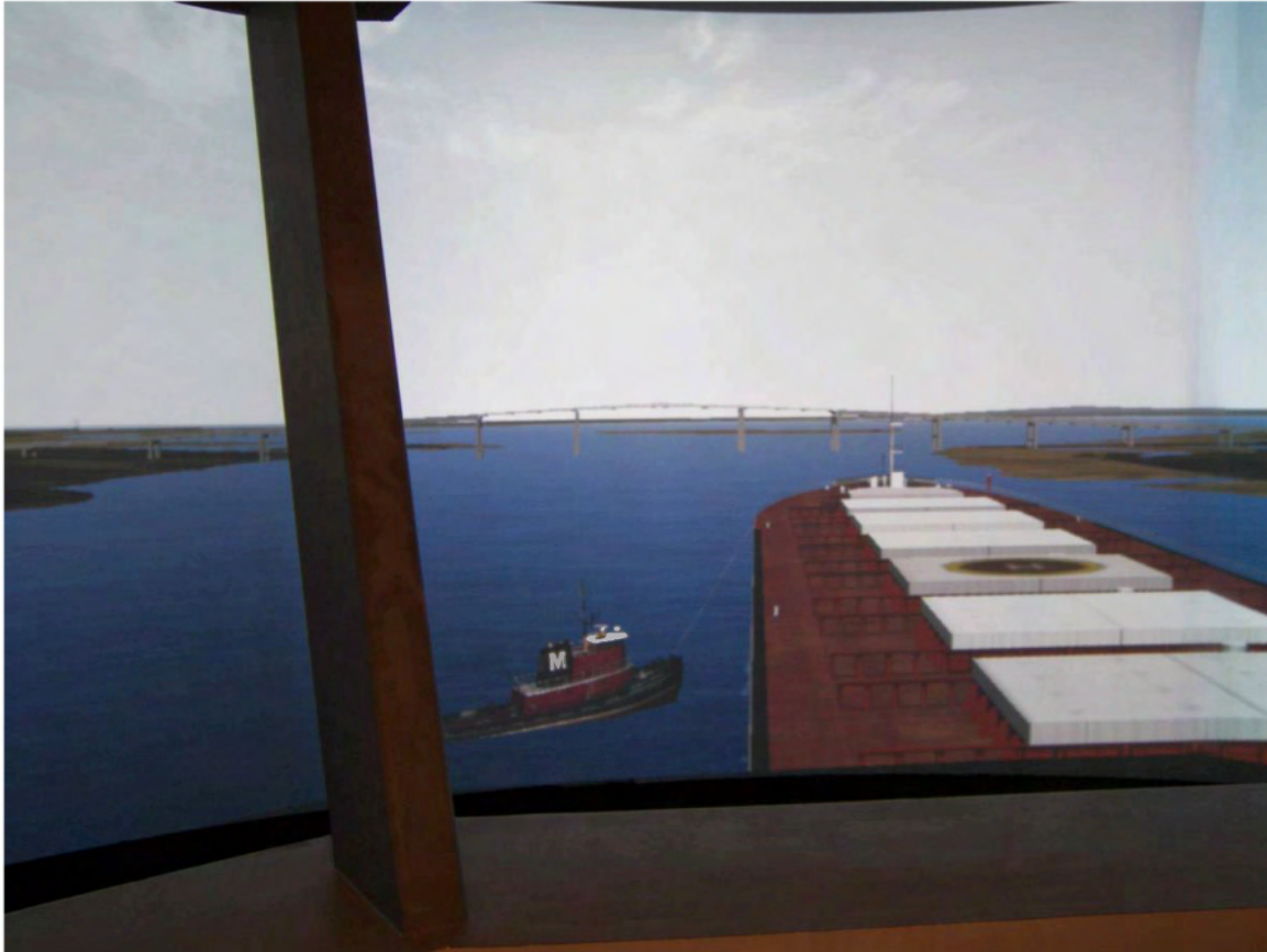
Figure 3: Simulation of a Bulk Carrier starting a 180 degree turn in the Samoa Channel turning basin, with the assistance of a 1600 horse power tug boat.
