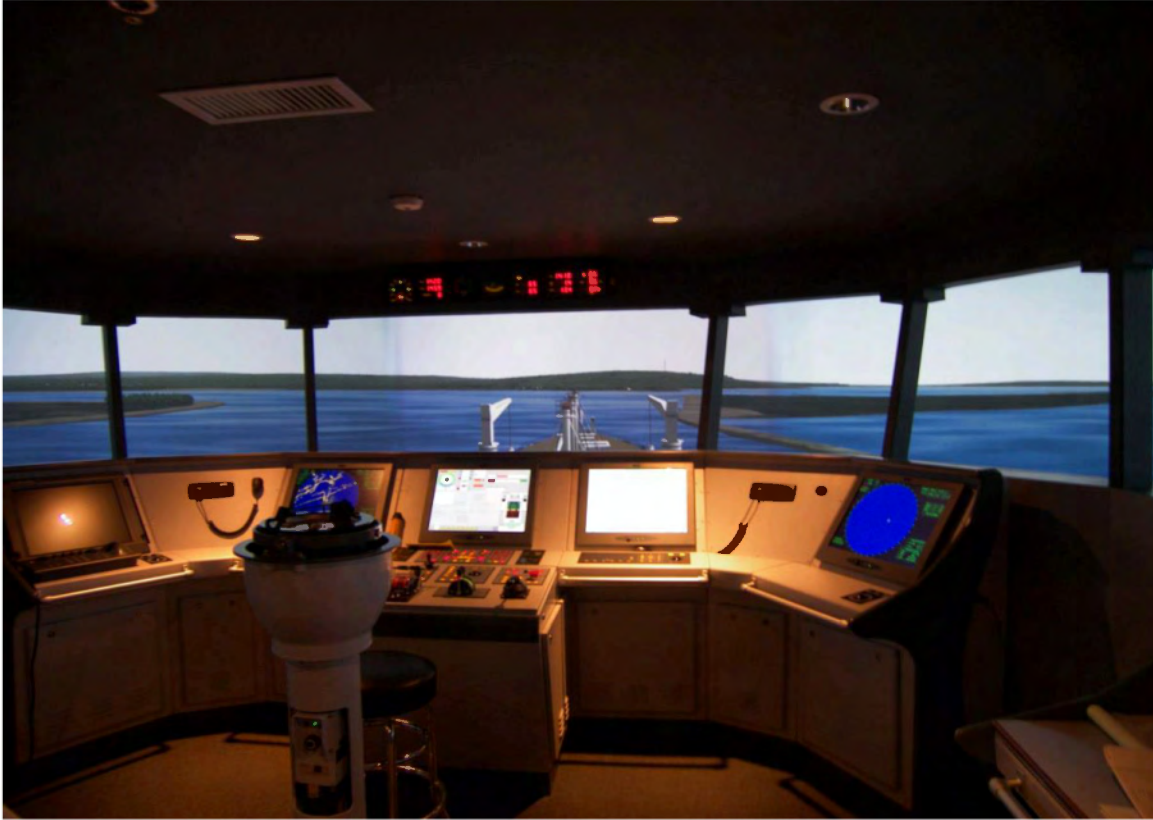
Figure 4: Simulation of a 1,132' LOA Tanker entering Humboldt Bay Entrance Channel.
